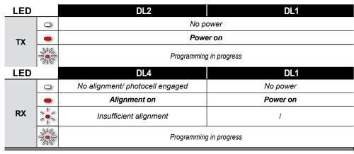
Words in bold: LED statuses with photocells powered, aligned and not engaged
