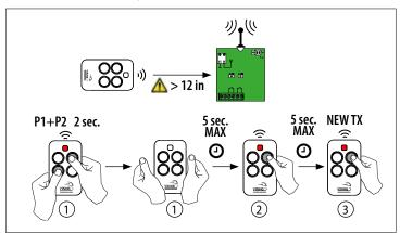
Adding new transmitters without accessing the receiver: Using a transmitter already stored on the receiver (1) press P1 and P2 for 2 sec. Release them. Press the push-button already stored (2). Press the button on the new transmitter that needs to be copied (3).
