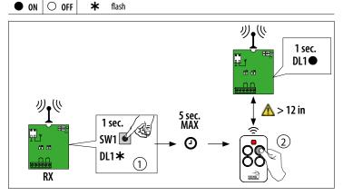
① Enable learning on the receiver: press SW1 for 1 sec. DL1 will start flashing ② Within 5 sec. press and hold the desired transmitter button until the receiver DL1 LED illumi
