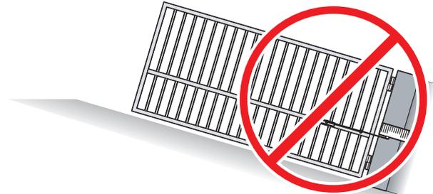
**DO NOT** install the gate operator to lift gates
