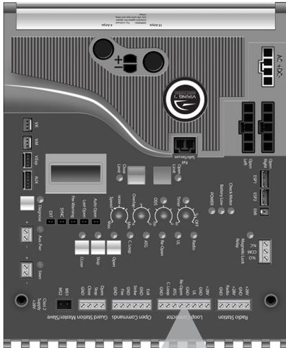
**NOTE:** The “Stop” LED will be flashing if there is a failure with at least one monitored entrapment sensor and the gate operator will be rendered inoperable.
