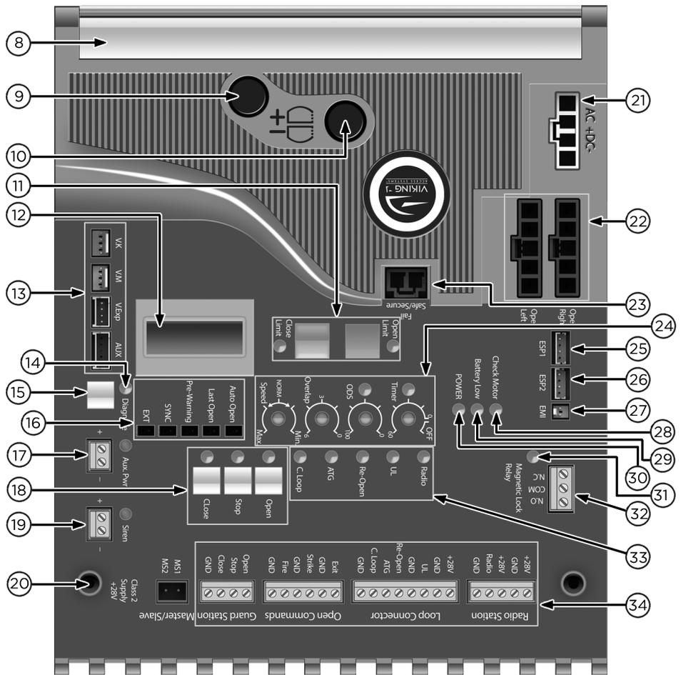
1. HEAT SINK - SECONDARY MODULE secures the control board and dissipates heat.
