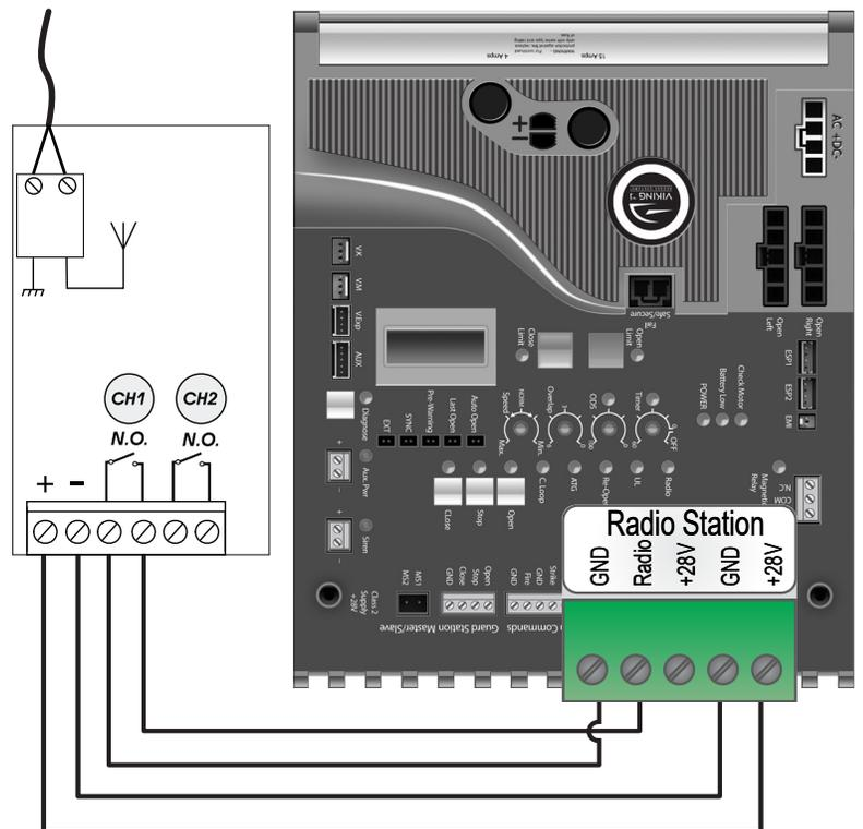
**⚠ TECHNICAL TIP:** The control board provides two modes of operation that a radio receiver can control the gate. For more information regarding accessory connections and terminal functions, refer to pages 28-29.
