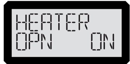
**NOTE:** If the application requires the gate to be held open for any reason, set the HEATER ON for both limit positions.
